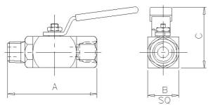
The 'B10' Type Single Isolating Ball Valve is designed for safe and reliable isolation giving bubble tight shut off. Totally enclosed soft seats offer both positive sealing and low operating torques, from vacuum to high-pressure service. Anti-blow out spindle is fitted as standard with the option of PTFE or Grafoil seals.
