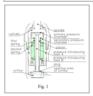
Refer to Figure 1 for design and operation of ASAHI AV Flow Control Valve. When the upstream fluid pressure, P<sub>1</sub> is introduced at the flow control orifice, it exerts a corresponding pressure on the upper surface of the flange on the piston type valve plug.
