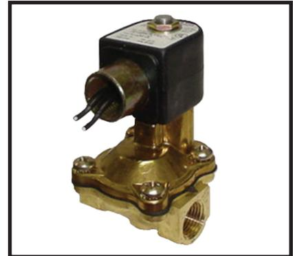
For best life and optimum performance, the Solenoid Valve should be mounted vertically upright, as illustrated in Figures 1 to 4, so as to minimize wear and reduce the possibility of accumulating foreign matter.
