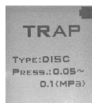
Steam trap automatic diagnosis mode screen
