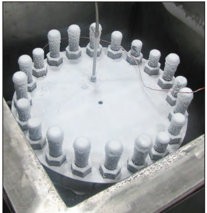
Dual-plate check valve after cryogenic testing.
