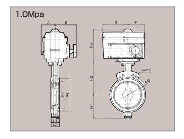
Dimension Table of JIS10K Specifications. Please contact us for sizes larger than 400A for JIS 16K flange.
