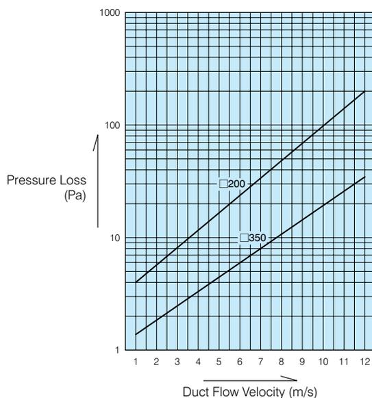
(Pressure Loss when HEPA filter final resistance of 0.4 kPa is applied)
