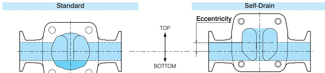
The valve seat is on the same centerline with straight pipe.
