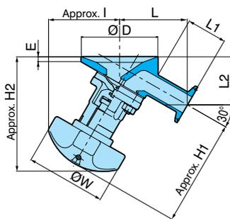
Pneumatically Operated ON-OFF Valve: BPO1414 (T) NB
