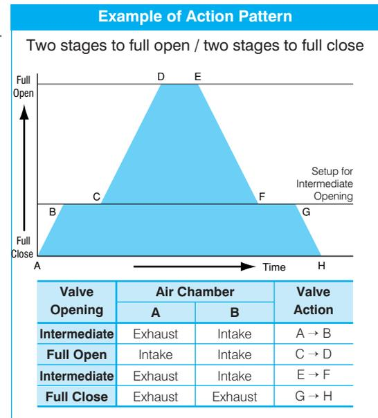
• Patterns “one stage to full open / two stages to full close” and “two stages to full open / one stage to full close” are available as well.
