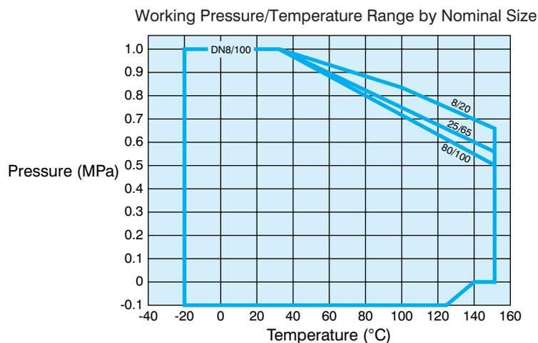
\* Lower limit temperature for PFA lined main body made of base material FCD-S is -10°C
