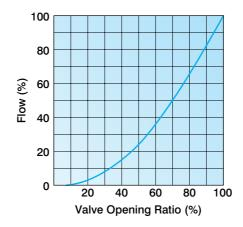
Flow Coefficient Cv Value (Adjusted Cv value considering rated Cv and effects by reducer)
