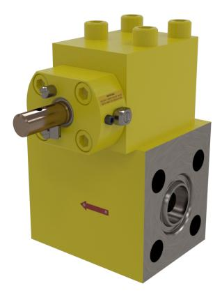
Image shown is a single Block 1" bore, half turn manual gate valve with 4 hole through bolted flange connections and integral 1" check valve. Due to the many options and configurations available with this product please contact Oliver Valvetek Sales for a bespoke solution.
