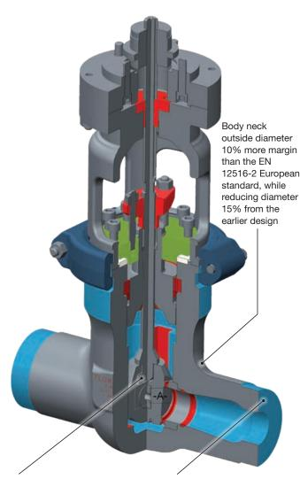
Gates, stem and seat ring designed to withstand requirements of higher allowable pressures of EN 12516-2
