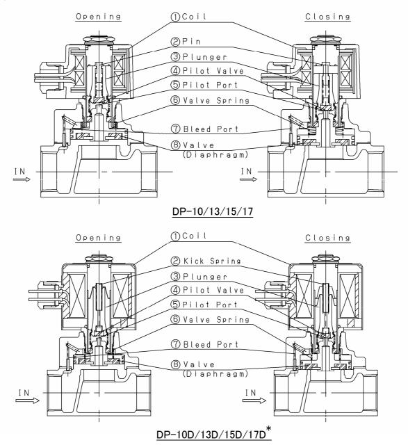
\* The structure differs slightly for DP-12/14/16/18/12D/14D/16D/18D.
