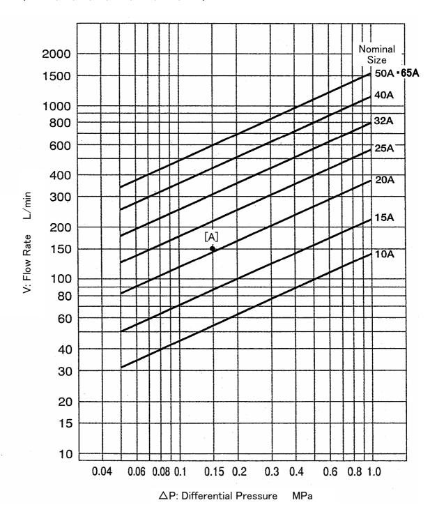
Under the following conditions, the appropriate nominal size would be determined as described bellow. Inlet pressure( $P_1$ ): 0.5MPa; Outlet pressure( $P_2$ ): 0.35MPa; Flow rate (V): 150L/min. First, find the point[A] where (V) and ( $\Delta P$ ) = ( $P_1$ ) – ( $P_2$ ). In the above example, the point[A] is located between the 20A and 25A nominal size valves, so the larger size of 25A should be selected.
