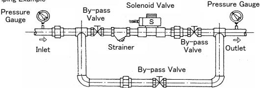
\* When the valve is used at 0.1MPa or less, mount the valve to the horizontal piping and the coil being at the top.
