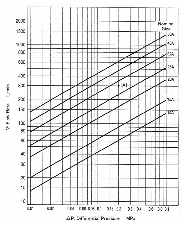
Under the following conditions, the appropriate nominal size would be determined as described bellow. Inlet pressure( $P_1$ ): 0.7MPa; Outlet pressure ( $P_2$ ): 0.5MPa; Flow rate (V): 300L/min. First, find the point[A] where (V) and ( $\Delta P$ ) = ( $P_1$ ) – ( $P_2$ ). In the above example, the point[A] is located between the 25A and 32A nominal size valves, so the larger size of 32A should be selected.
