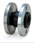
RUBBER EXPANSION JOINT WIDE ARCH DESIGN. SINGLE SPHERE WITH SS41 FLANGE TO ASA 150 LBS, DIN PN16, DRILLED. VACUUM 26" HG. SIZE: 2"~16"
