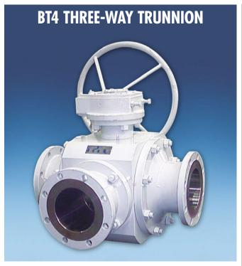
Three-way (three port) trunnion mounted ball, split bolted body, anti blow-out stem, antistatic device, and fire safe design
