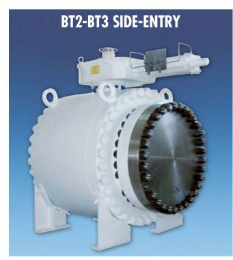
Two- or three-piece split bolted body, side-entry trunnion ball valve with anti blow-out stem, antistatic device, and fire safe design
