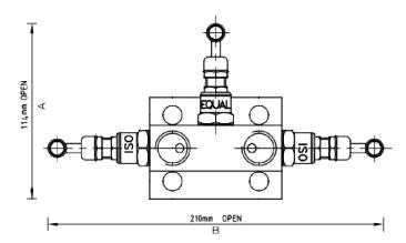
The 'T34' Type 3 valve manifolds are designed for direct mounting to differential pressure transmitters, with separate isolation for LP and HP inlets plus equalising valve for simple calibration. Each needle valve head is designed for safe and reliable isolation, giving bubble tight shut off, with non-rotating & anti-galling tip and dynamic self-adjusting spindle seal to give long service life in a variety of service conditions.
