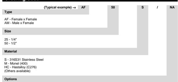
AG - Grafoil AT - Anti-Tamper HL - Handle Locking HL-PI - Handle Locking + Position Indicator
