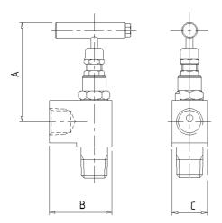
The 'A' Type Single Isolating Needle Valve is designed for safe and reliable isolation giving bubble tight shut off, nonrotating & anti-galling tip and dynamic self-adjusting spindle seal to give a long service life in a variety of applications.
