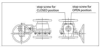
Fig. 14 Open and closed positions of the M actuator
