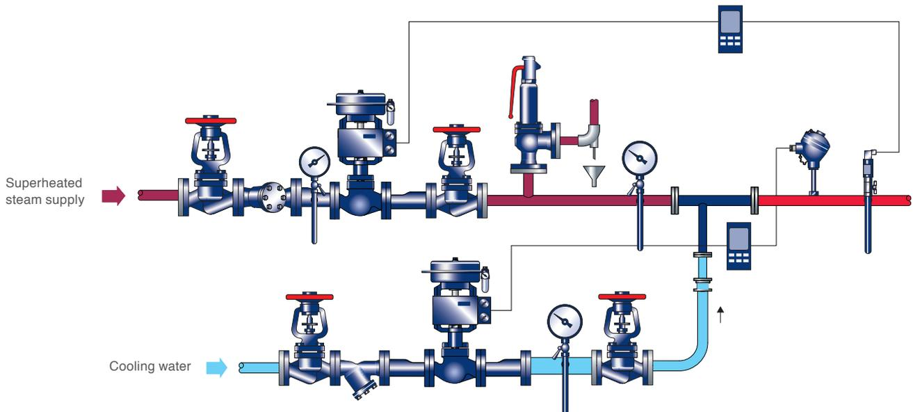
The above overview shows a typical pressure reduction and desuperheating station installation including a pressure control valve, a temperature control valve and a desuperheater. Each ancillary component of this installation ensures the longevity and proper operation of the control valves and the desuperheater.
