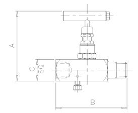
The 'GB' Type Gauge Bleed Needle Valve is designed for safe and reliable isolation, giving bubble tight shut off, with non-rotating & anti-galling tip and dynamic self-adjusting spindle seal to give long service life in a variety of applications. The additional ability to bleed the gauge cavity to atmosphere, for simple calibration, is included.
