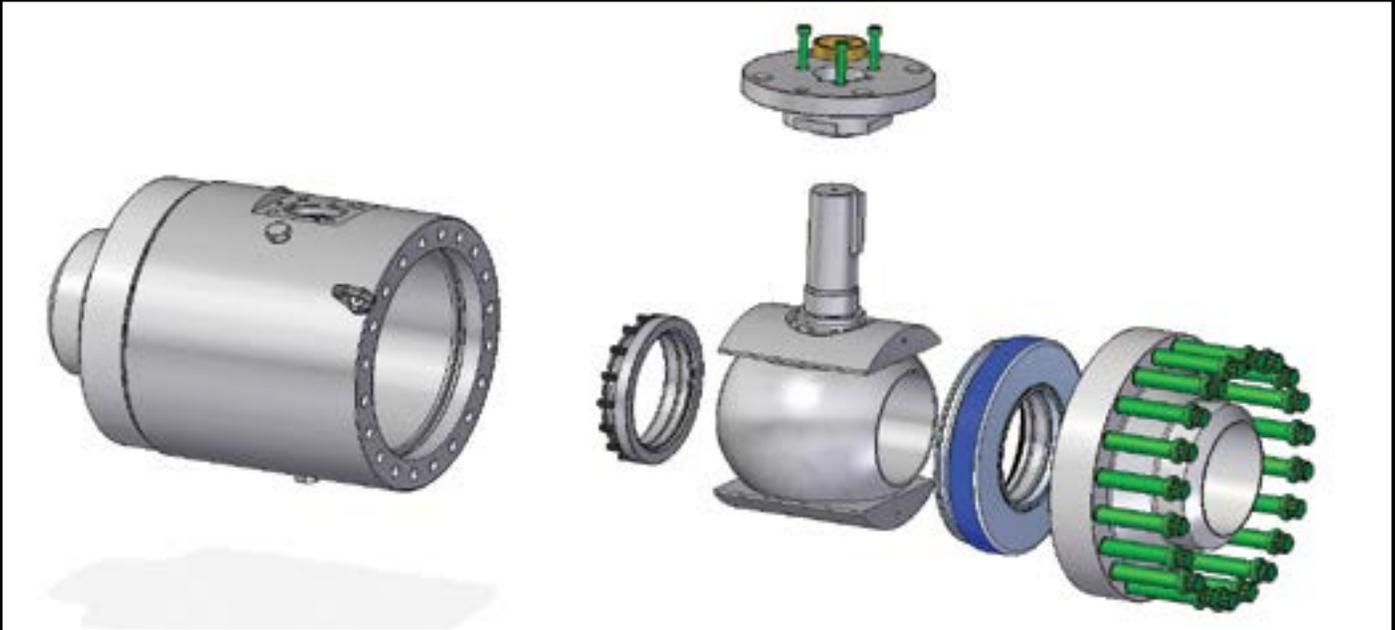
*Perar Compact Ball Valves are designed according to API6A to combine a compact design with robustness and reliable performances. The valves do not rely on lubricant or grease to assist sealing between the ball and seat also when metal-to-metal sealing is used. The valve design is based on trunnion mounted or support plate configuration in order to get the operating torque as lower as possible.*
