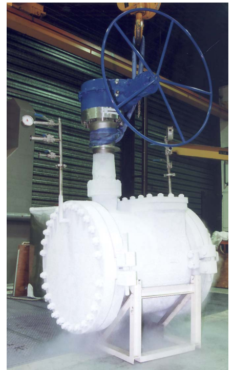
42" BW Side Entry Butterfly Valve after cryogenic tests
