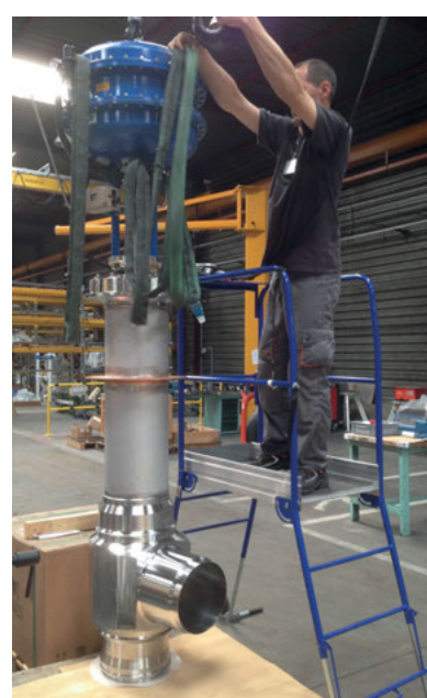
Angle control valve size ND250 with thermal collar
