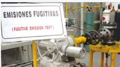
**Low Fugitive Emissions Test.**- When a Customer requires low fugitive emissions certification, the Lab has its own LFE Test Equipment capable of measuring less than 20 ppm in either static or mechanical conditions at ambient temperature or thermal cycle operations.
