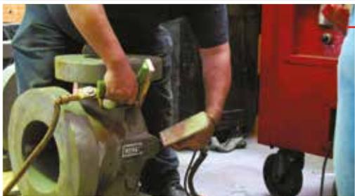
**Magnetic Particle Test.**- On a random basis for standard products or when a Customer requests MT Certification, WALWORTH uses Magnetic Particle Testing Equipment on ferromagnetic materials.
