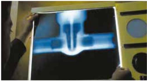
**X-Ray Examination Equipment.**- WALWORTH has its own Ir-92 source in-house for the radiographic examination (RT) of castings from 0.100" up to 2 1/2" wall thickness to verify the soundness of the raw casting material.
