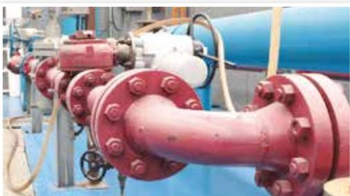
**Test Loop.** A complete Laboratory Test loop exists for design validation of WALWORTH products, performing the test at maximum design pressure and cycling the valves from 3000 to 5000 cycles. The test takes more than four months to be completed.
