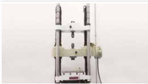
**Tensile Test Equipment.**- To verify the mechanical properties of materials used for manufacturing, WALWORTH tests samples on a random basis even though we receive MTR's from our suppliers and foundries.
