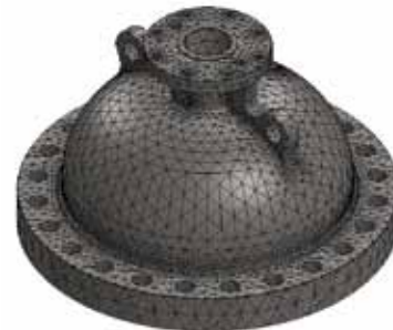
FINITE ELEMENT MESH USED IN OPTIMIZATION STUDIES
