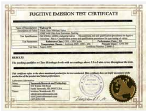
Emissions after 500 cycles at ambient and 350 °F Issued by Yarmouth Research and Technology Lab for 3 inch Class 300 Gate Valve After 500 cycles the measurement result was less than 50 ppm.
