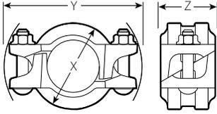
Rated for wet and dry sprinkler systems at 350 psi/2413 kPa for 1 ¼ – 4”/32 – 100 mm sizes and 300 psi /2068 kPa for 4 ¼ – 8”/108 – 200 mm sizes; Schedule 10 roll grooved or Schedule 40 cut or roll grooved steel pipe. Style 005H is rigid and does not accommodate expansion, contraction or angular deflection.
