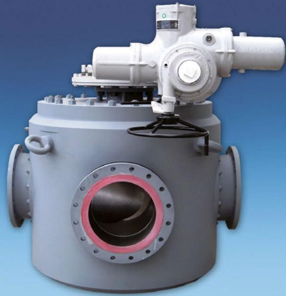
Four-way double “L” port diverter valve suitable for changing flow directions with special design for avoiding the stop of the flow
