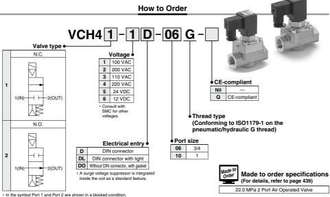
In the symbol Port 1 and Port 2 are shown in a blocked condition, but it is not possible to use the valve in cases of reverse pressure, where the Port 2 pressure is higher than the Port 1 pressure.
