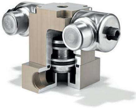
The Scram Solenoid Pilot Valves (SSPVs) are an integral part of the BWR reactor protection system. SSPV type 2562 was designed to original specifications and fits into the existing mounting configuration of the BWR Hydraulic Control Unit with no hardware modification needed.
