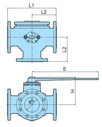
This valve is not compatible with E300NB-L2 in face to face dimension and parts.
