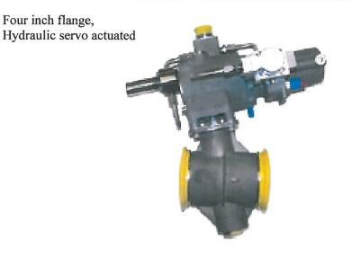
Meggitt's butterfly valves are designed for bleed air control on aero-derivative industrial gas turbine engines. This design was generated specifically for increased cycle life of the bearings and butterfly element while implementing precision control and position indication.
