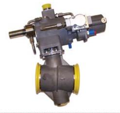
Meggitt's butterfly valves are designed for bleed air control on aero-derivative industrial gas turbine engines. This design was generated specifically for increased cycle life of the bearings and butterfly element while implementing precision control and position indication.
