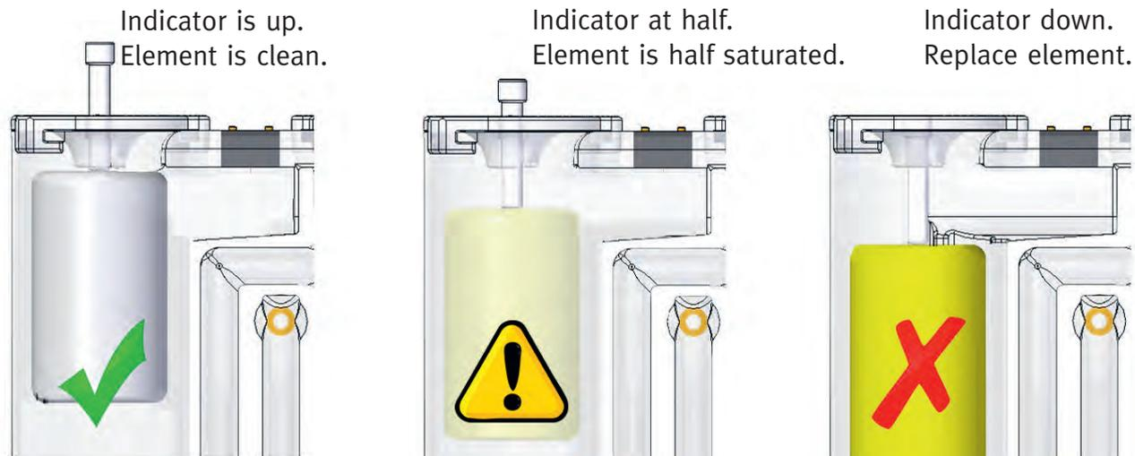
One unique feature of the SEPREMIUM separators is the element life indicator. This indicator gives instant visual confirmation of the condition of the elements in the separator and when they need to be replaced.
