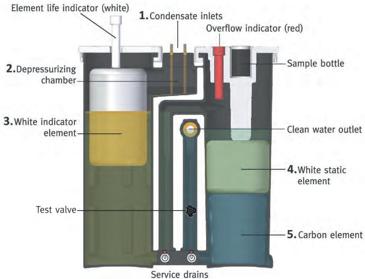
1. Condensate enters the brass condensate inlets. Unlike traditional separators which require the use of zero air loss drains to reduce emulsification, the SEPREMIUM can accept, and effectively separate, virtually any condensate from any source using any type of drain.
