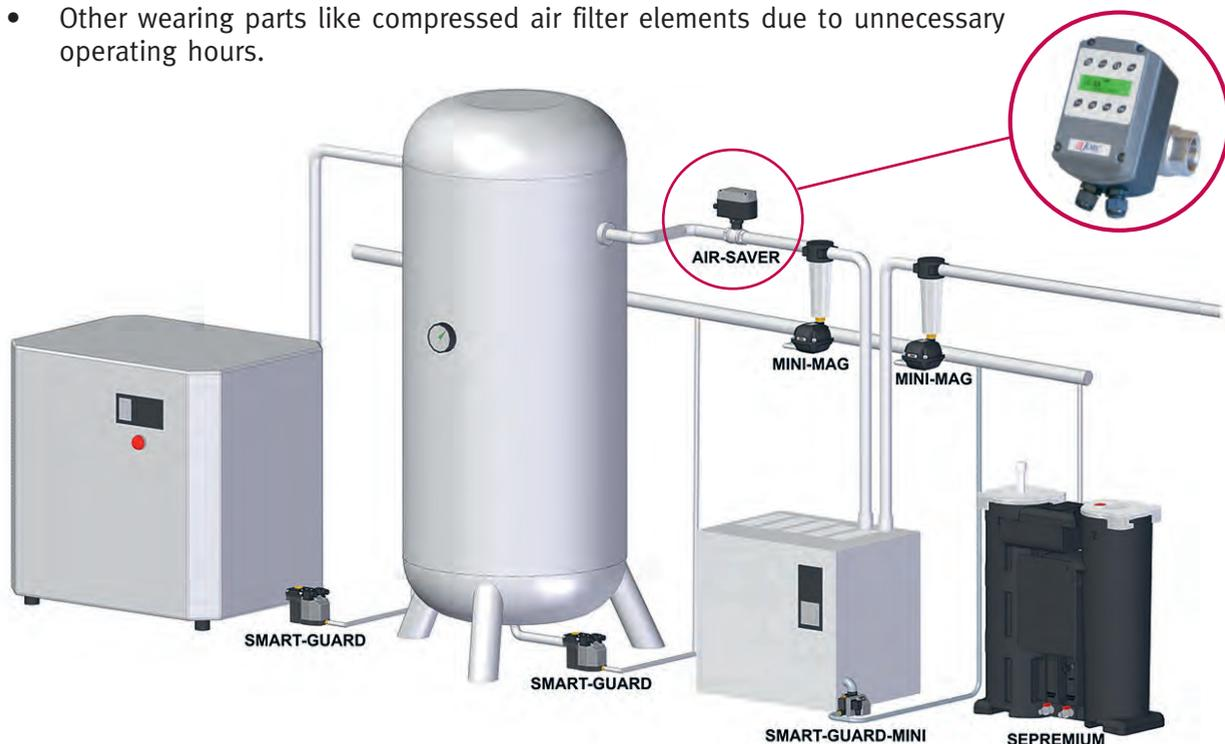
**GRAPH A: COMPRESSED AIR SYSTEM WITHOUT AN AIR-SAVER**
