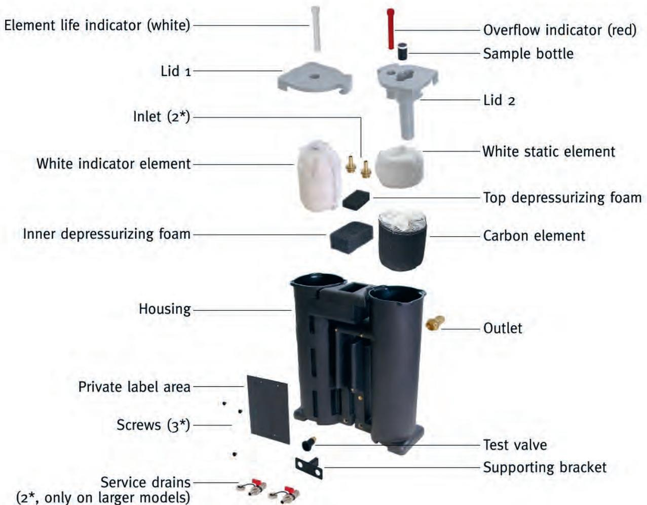
The SEPREMIUM 350 up to 2500 models are equipped with double service drains for quick and easy service options.
