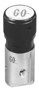
The CPR-1 Series is a compact pressure regulator with most of the same internal design features employed in our time proven PR-1 Series. This regulator was designed to provide optimum performance as a "lecture bottle regulator" for pressure control in any application where a small size and low internal volume are required. The low internal volume allows more rapid purging in analytical instrumentation and semiconductor doping gas applications.
