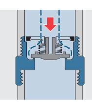
Pump stationary, SBO preventing gravity circulation
