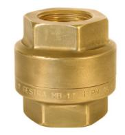
MB 14 Screwed 1/2-2"BSP. body material hot-pressed brass, valve disc of austenitic steel
