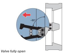
The rotary movement of the plates is limited by stop lugs to 80°. Additional hinge stop lugs ensure a stable position of the plates when fully open.
