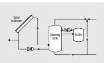
Preventing backflow protects the pump against backflow after it is switched off
