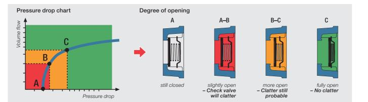
Degree of opening of a spring-assisted check valve as a function of volume flow
