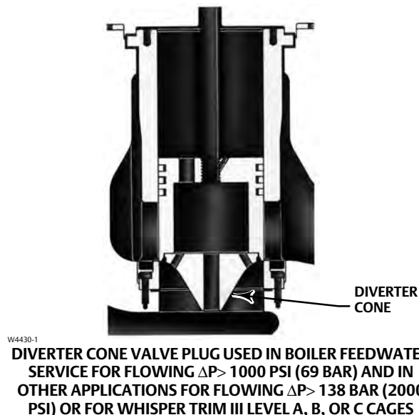
Figure 12. Diverter Cone Valve Plug Used in Fisher EHD and EHT Valves (NPS 8 through 14 Globe Valves, Flow Up Only)
