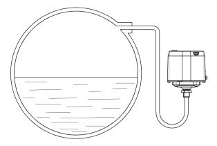
The pressure switch can be mounted in any position, but the mounting with vertical axis and pressure intake as per scheme is suggested. This to avoid that the boiler deposits obstruct the pressure pipe.
