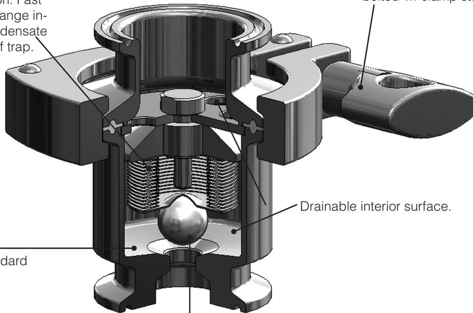
Ball type tip helps insures low subcooling operation by providing maximum flow with minimum lift. Helps insure minimum condensate backup upstream of trap.
