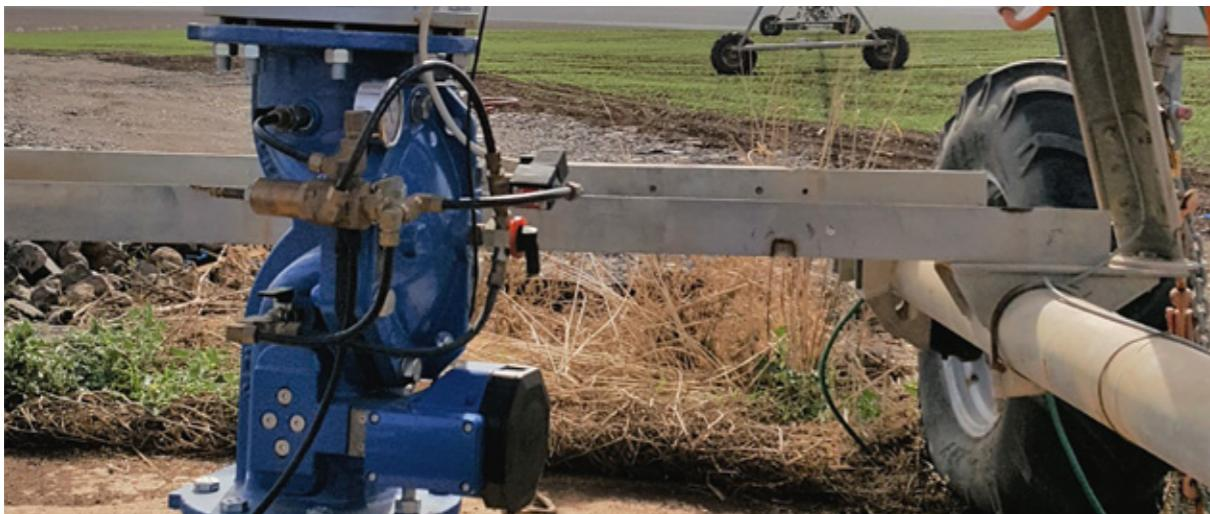
Ultraf Ultrasonic Hydrometer installed on the Pivot
