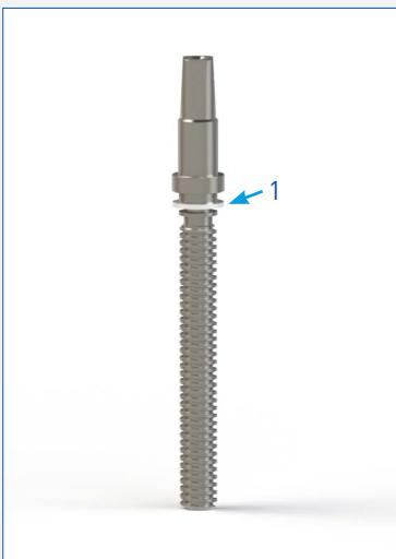
**04:** Stem and collar made in one piece in stainless steel for **better resistance to axial load and to withstand higher operating torques**. A polyamide washer (1) placed under the collar allows to reduce friction torque and protect coating inside the Bonnet.
