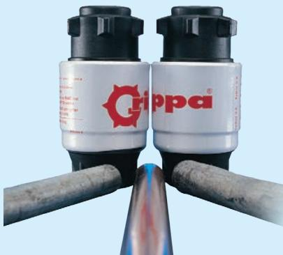
The Talbot Grippa is a universal fitting that connects onto a wide variety of existing lead, galvanised iron and copper pipes with no change of components. The range consists of just three fittings which suit all metal pipes with outside diameters of 15mm ( $\frac{3}{4}$ ") to 34mm ( $\frac{3}{8}$ ").
