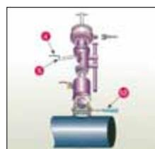
**4** When drilling is finished, the automatic feed is switched off by loosening screws (4) and (5). The drilling ring is taken out of the pipe, bearing in mind that if the hole has been drilled on a working-pipe intake ring, the water inlet must be closed either by means of the spatula or the valve (12).
