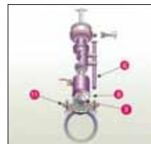
**2** The drilling ring (9) and the adjusting nut (8) are fixed onto the machine, and the machine onto the saddle (11) by inserting the anti-rotation bar (6).
