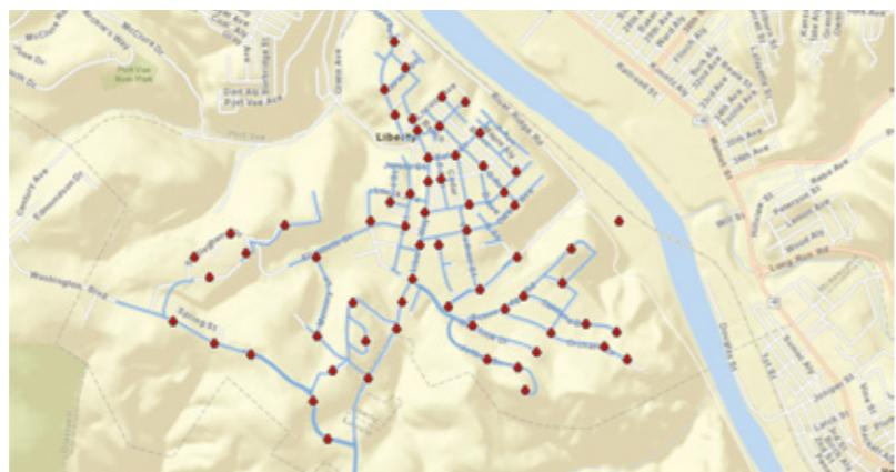
Network with fire hydrants equipped with EchoShore®-DX modules.
