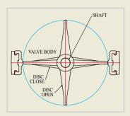
The valve shall be a 90° turn clockwise to close, non-jamming, and resilient seated valve for zero leakage service.
